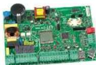
High efficiency MPPT charge controller optimized for LiFePo
