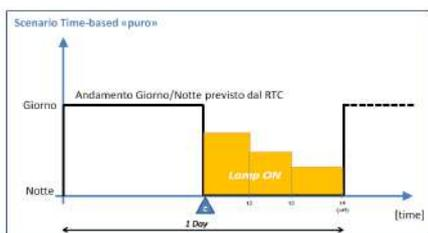
Figure 4 - Example of Time-based working mode
