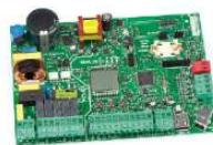
High efficiency MPPT charge controller optimized for LiFePo and NiMh batteries.
